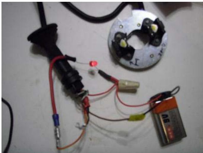
Insert a thin bit of steel to interrupt the field. Don't tell SWMBO I used the butter knife. Light goes off. Upper trigger is good at room temperature. Test it later after heating with a hair dryer. If it lights up when uninterrupted, and goes out when interrupted, it's good. If not, failure under heat. No good.
