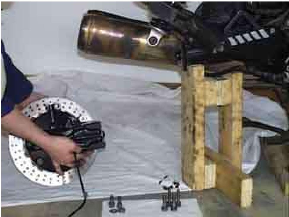
...at which point the drive is totally free and can be laid down flat (on the rotor). Gear oil should not be able to leak out in this position.
