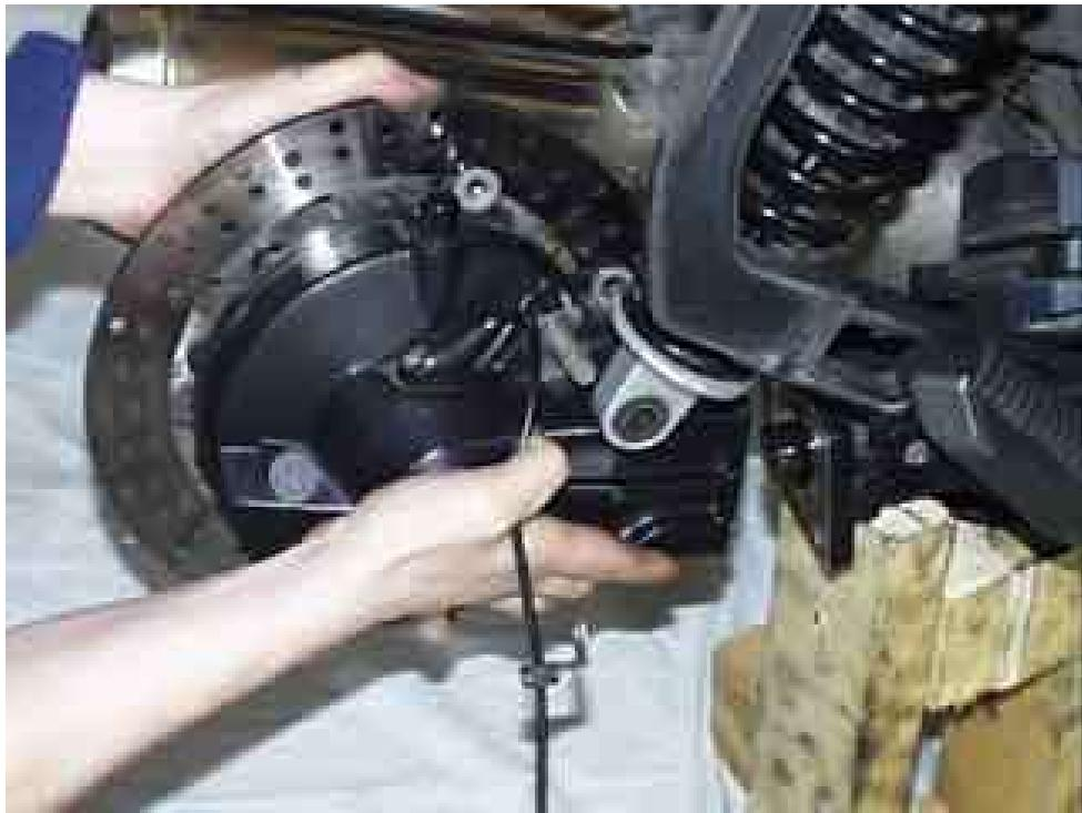
When it is free of the swingarm, pull it backwards a few more inches (to disengage the driveshaft) and then move it to the left to unhook it from the shock...
