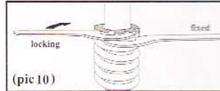
Using small screw to lock or unlock the spring preload
