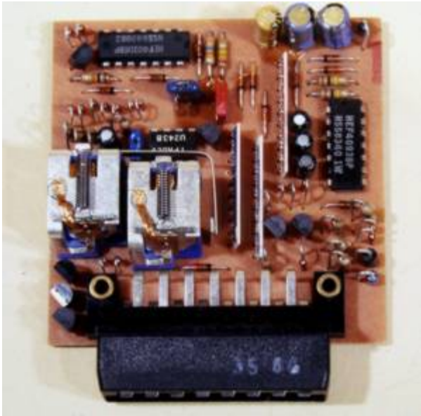
Above: The indicator board with relay prevents voltage drops
