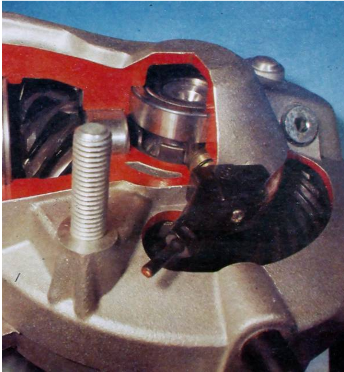
Above: Speed and distance measurement on the K75 and K100 is carried out electronically with an inductive sensor.
