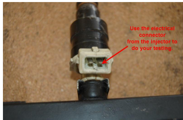
Testing the coil of the fuel injector
