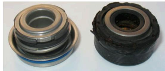
New mechanical seal to the left, the old type to the right.
