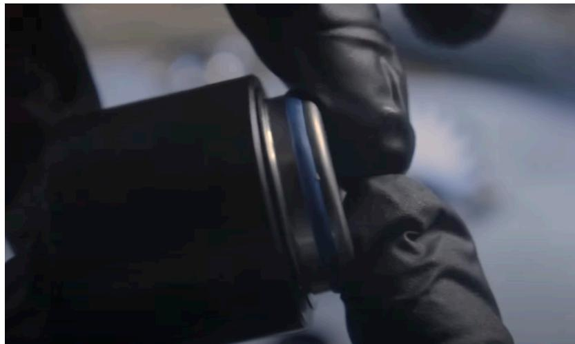
The seal is pressed or punched in place over the shaft.
