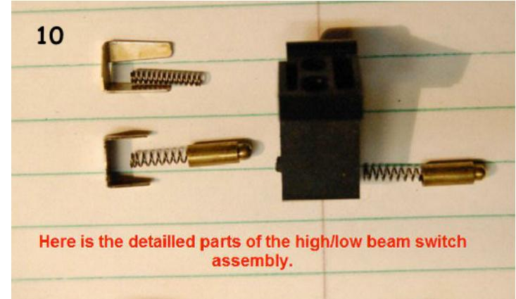
Here is the detailed parts of the high/low beam switch assembly.
