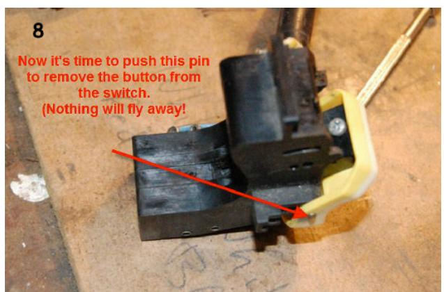
Now, put the switch in a clear plastic bag and pull the rotating part out of it. Springs may fly away!!
