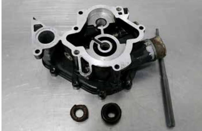
Lubricate the lip of the new oil pump seal with and drive in with an appropriate socket
