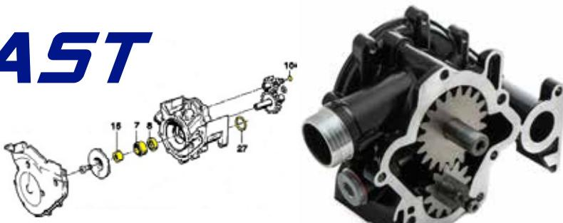
First drive out the old water pump seal then the oil pump seal and clean out the bore for the seals.
