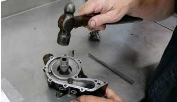
Install the oil water pump shaft. Place assembly in a press, use the specially designed press tool to push the seal into the housing **and** onto the shaft at the same time. Back the large gear in the press, Best to accommodate the shaft to pass through the bottom of the press.
