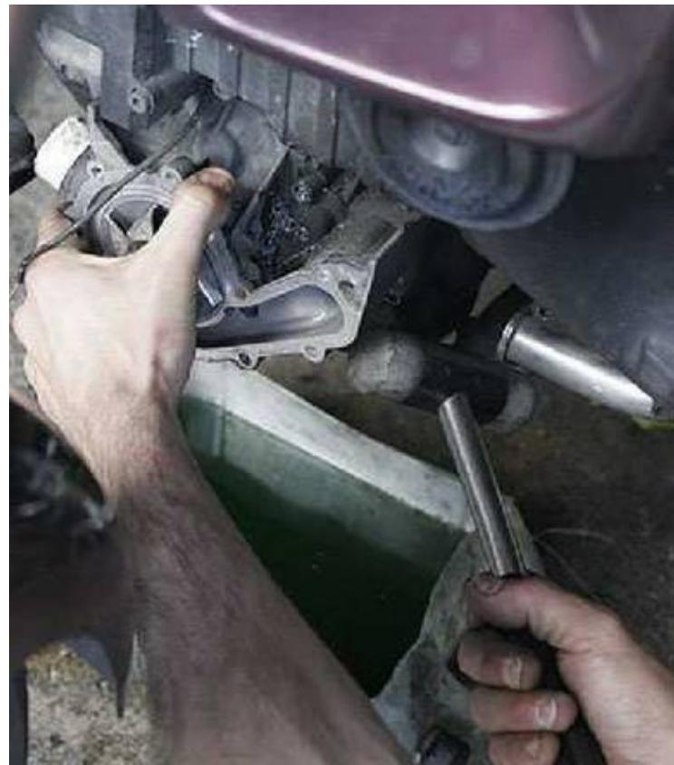
**The pump is now removed, and because of the front wheel being lifted, you will lose only the equivalent of a glass of oil**
