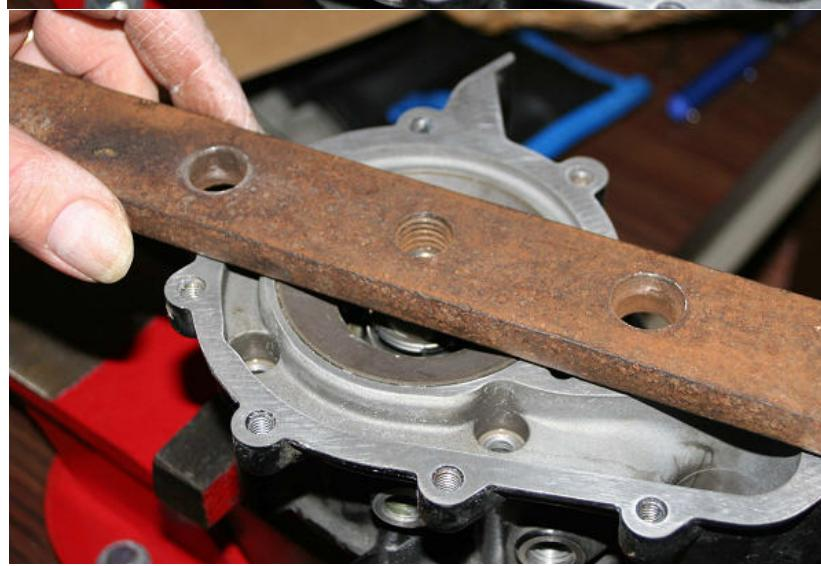
**Install the new spacer then the turbine and torque the screw to 3.3kg/nm.
