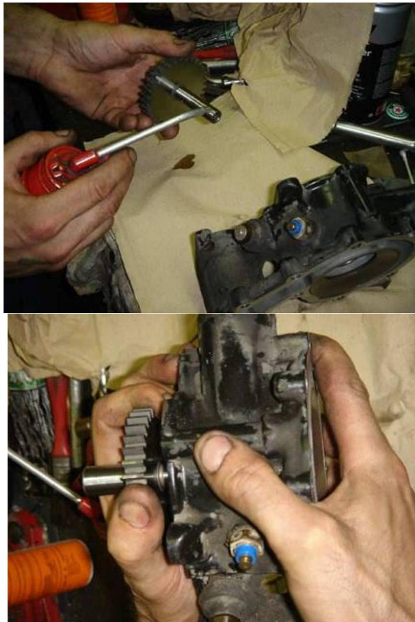
**To pull the shaft, we will use an 8mm threaded road, a nut and the old spacer.
