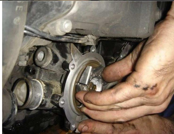
**Put some gasket sealer on the water pump cover, re-install it
