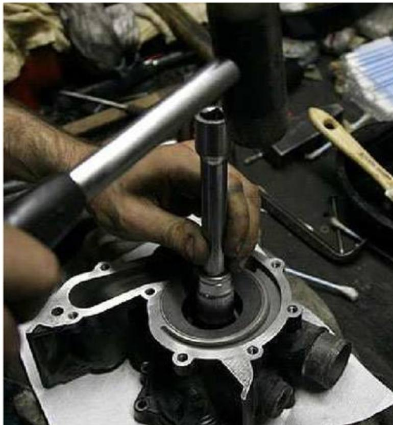
**The water seal is inserted the same way as the oil seal but using a 27mm socket.
