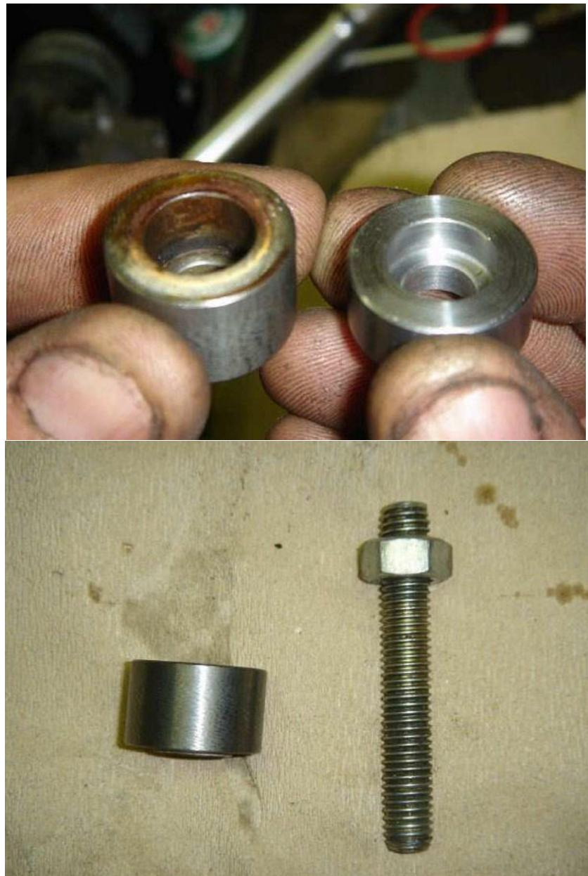
**Screw the threaded rod onto the shaft, put the spacer (or the 19mm socket + the washer), the nut and pull the shaft until the gear comes flush with the casing.
