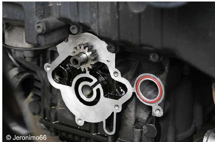
**Put some gasket sealer on the pump housing (Not too much near the gears), put the pump in place turning it to match the teeth on the pinions.**
