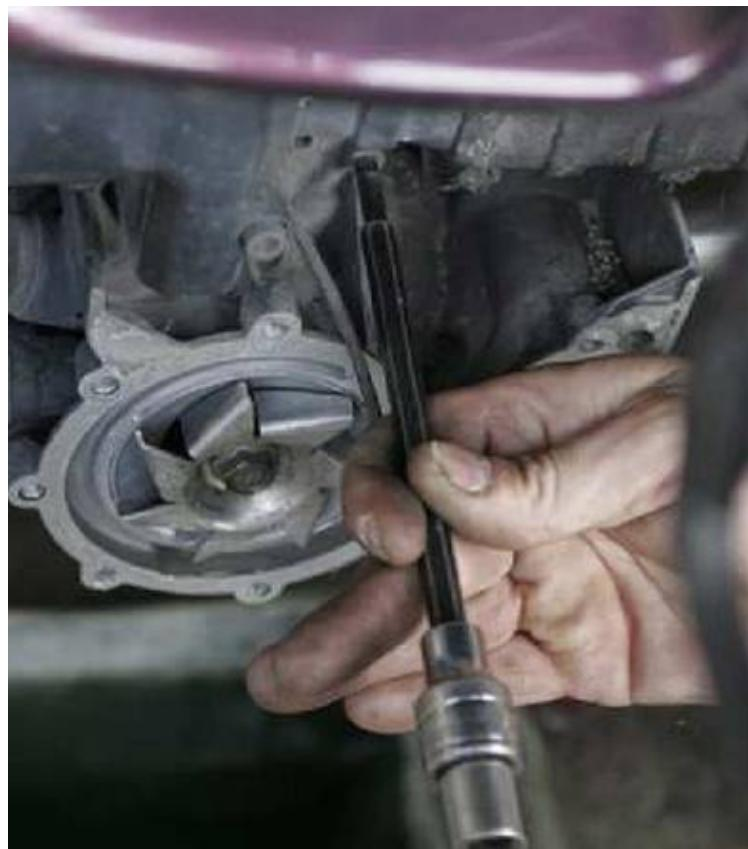
**Put a container under the pump to catch the oil.
