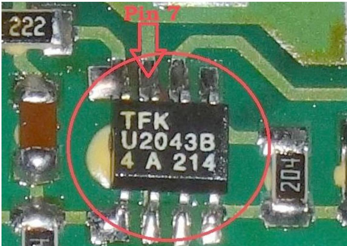
How I did it: For the black flasher relay I used the tip of a pushpin to break Pin 7 and bend it up and out of the way.
