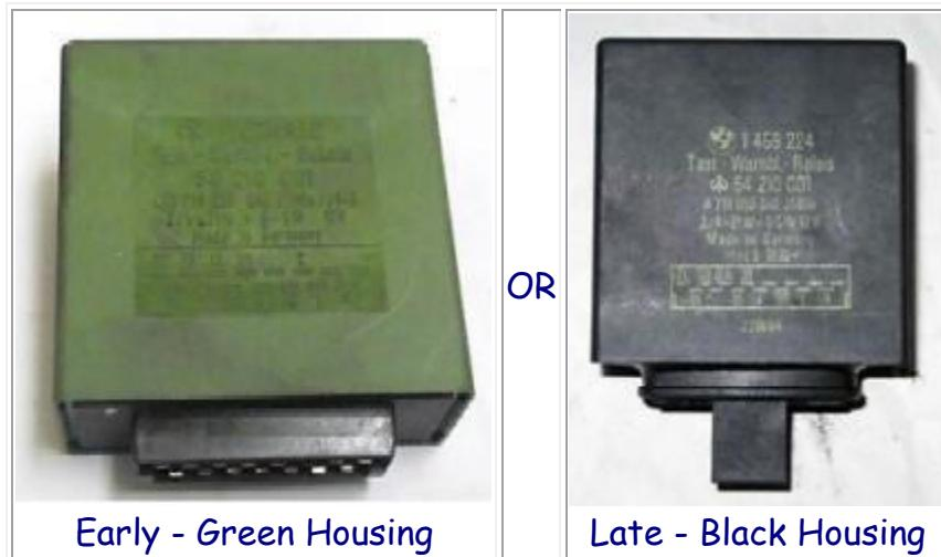
Despite the different colored housings, they are the same part (61311459224) and are interchangeable. Although they operate exactly the same, the circuitry inside them is slightly different. Click the thumbnails below to see the details.
