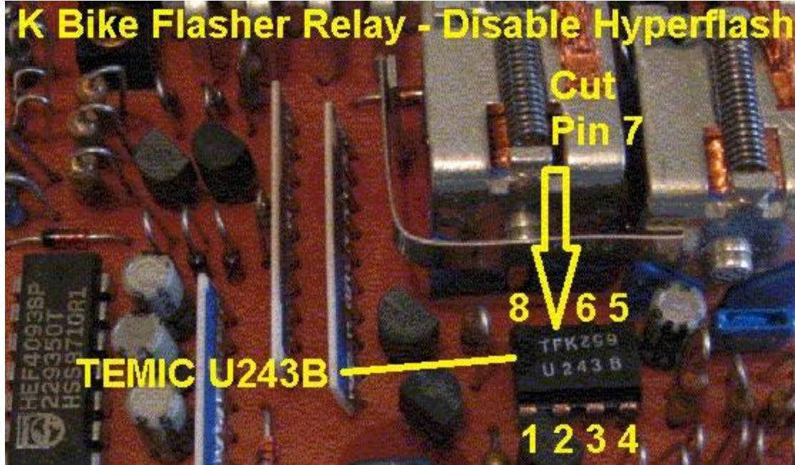
How I did it: For the green flasher relay I first pushed the U243B chip towards the 1-4 pins to make 5-8 more exposed. Then I used a small screwdriver to pry Pin 7 up out of the circuit board and bend it out. I then used some small diagonal cutters to cut off Pin 7.
