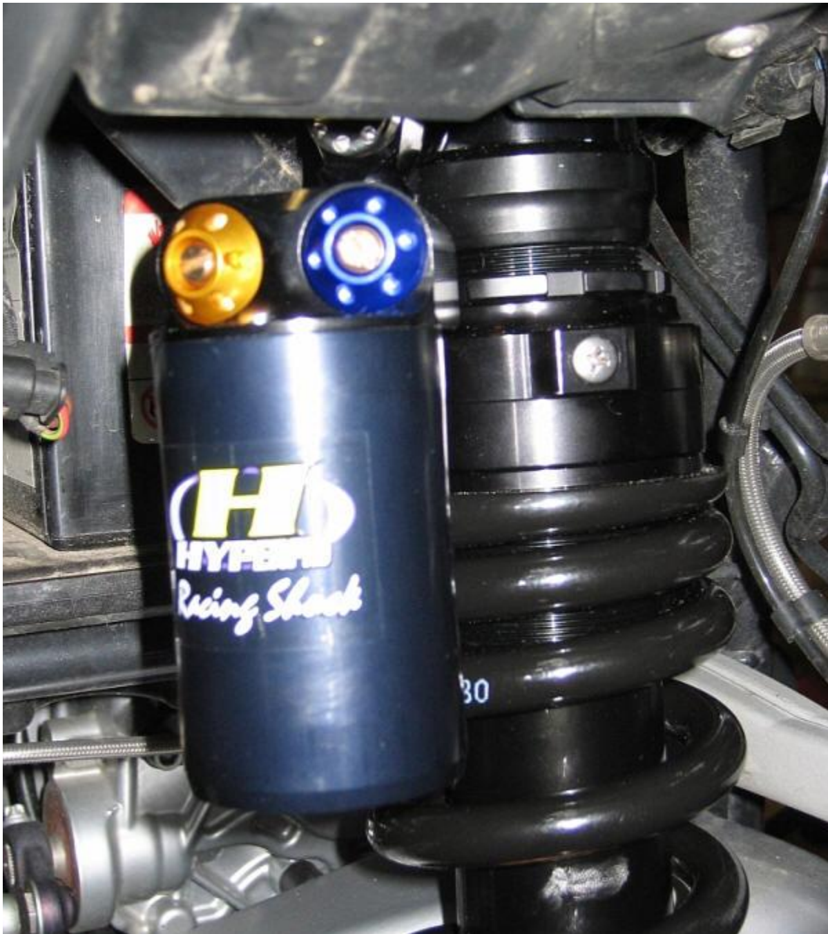
Blue and Gold rings surround the low and high speed compression damping adjustment on a Hyperpro shock
