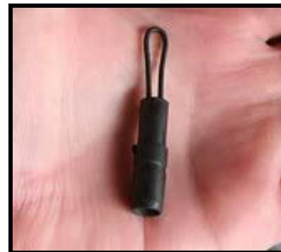
The altitude plug is BMW part # 61 13 1 459 504. All it is is a loop of wire that shorts two leads. I usually wire it up to a dash switch because stopping to insert or remove a plug seems kind of dumb to me.
