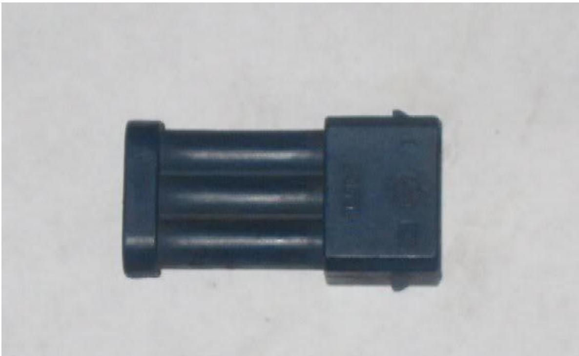
Once you've located the diagnostic plug cap, remove the cap and stick the stripped end of a piece of wire into the center terminal of the diagnostic plug. Ground the other end somewhere on the bike. For 93 and earlier K bikes a good place to ground the other end of the wire is where the battery ground is bolted to the left side of the transmission near the shift lever.
