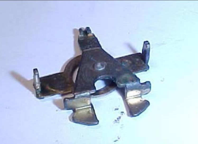
7. The contacts AFTER cleaning and polishing. The fixed contacts should also be this clean.
