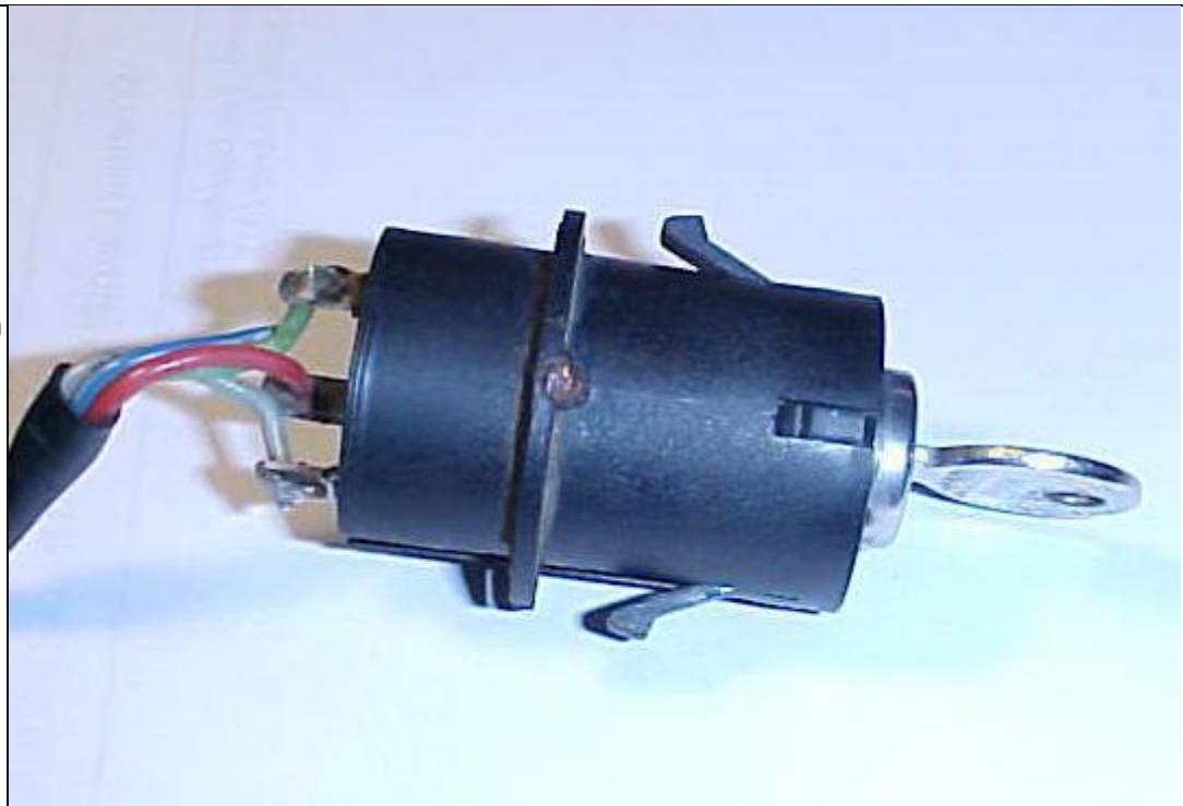
2. Disassemble the switch from the cylinder/barrel assembly. You can clearly see the backed out setscrew in this photo. It goes into the round hole on the white part of the switch shown in this photo on reassembly.
