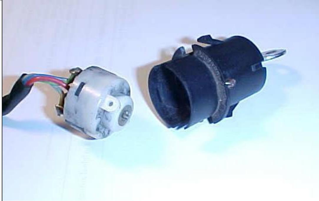
3. The retaining tangs (there are two of them) that hold the switch together.
