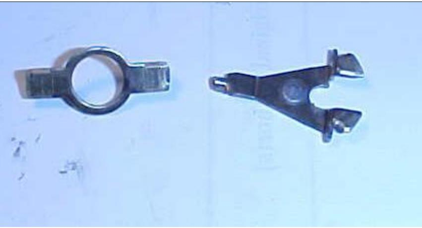
8. Reassembly - use some good quality grease on the contacts before reinstalling them. A small smear (tech-term) is more than enough. Too much is not a good thing.
