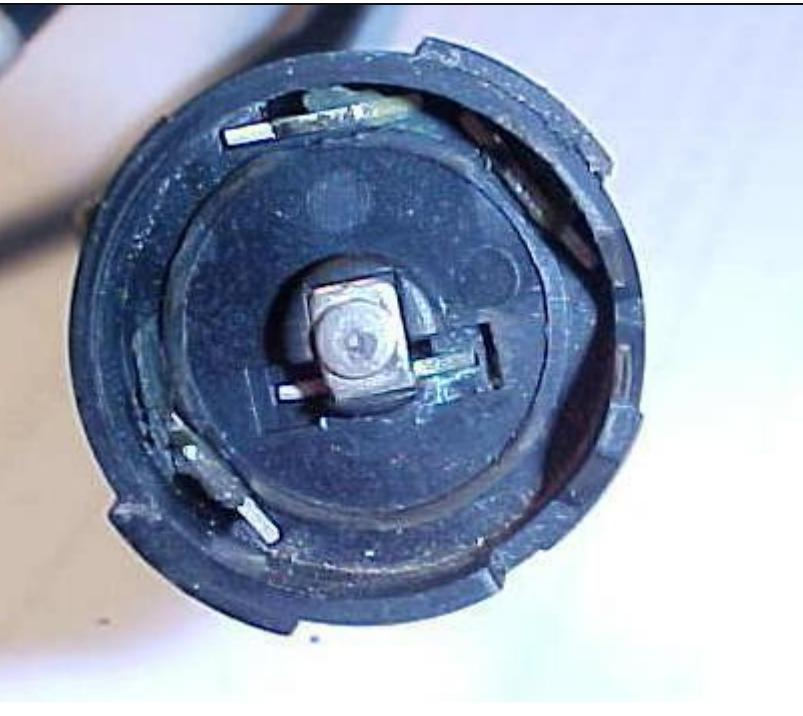
6. The rotating contacts - again - the goal is to get these nice and clean with no signs of burning on the contact surfaces.
