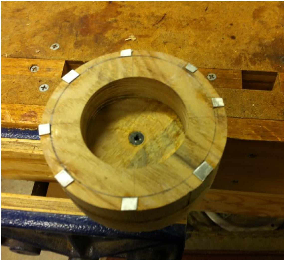
If you plan on using wood, use something hard like oak or ash. I used ash. After I drove the seal on it was slightly cocked so I tapped on the driver around the circumference to seat it evenly.
