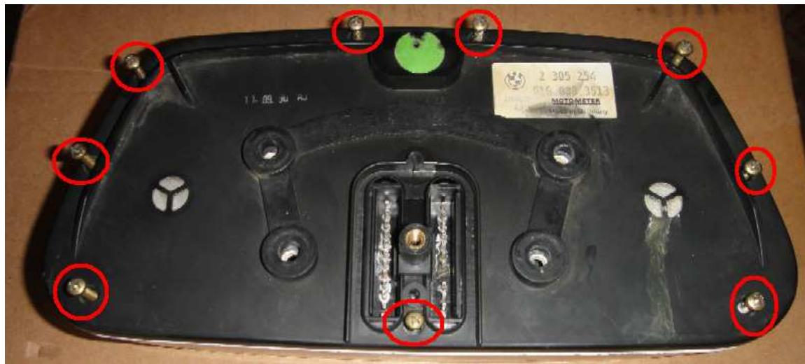
Then remove the six Phillips screws that secure the “guts” to the front housing.
