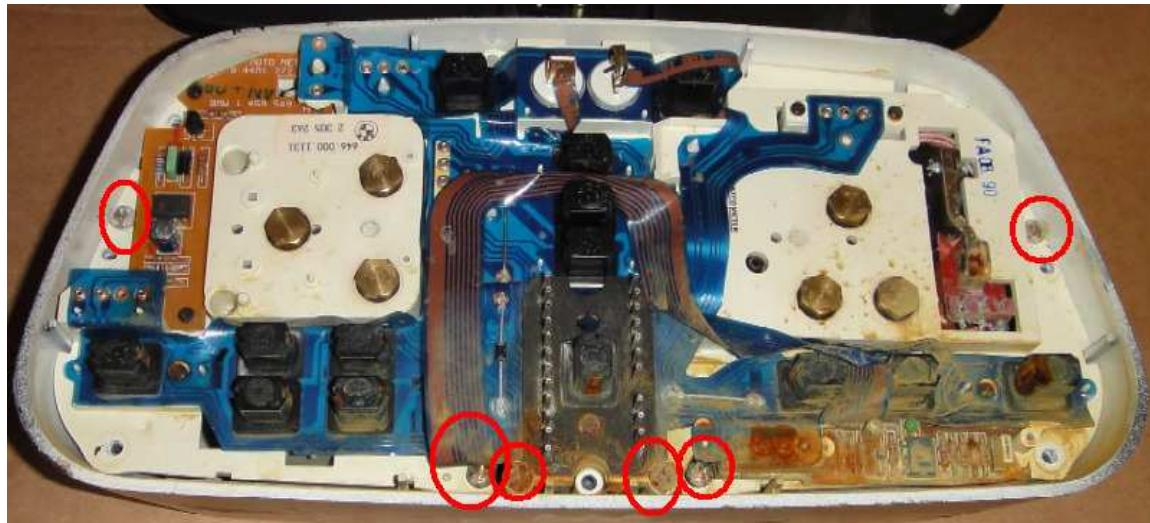
Now turn it over, pull the trip odometer knob out about 1/4" and carefully shake the guts out of the housing. The trip odometer knob does not need to be fully removed as there is a notch cut out of the speedometer faceplate for it to pass through.
