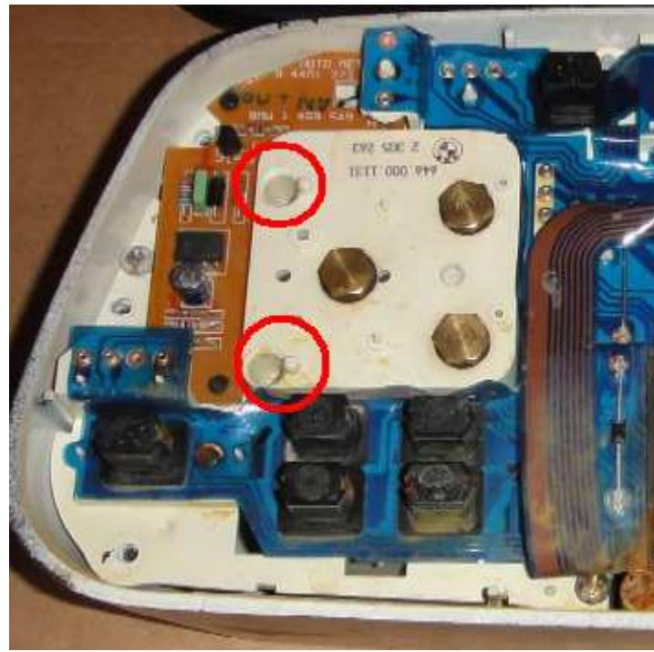
Once those screws are removed, you can remove the white plastic spacer from the side.
