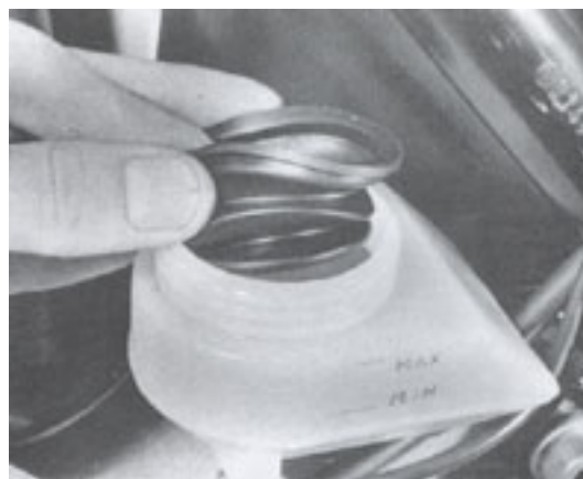
Ensure diaphragm is clean and dry before refitting
