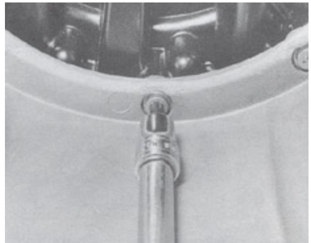
7.7b .... Torx type - special key required for removal and refitting
