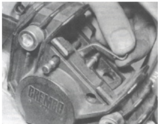
..... insert first retaining pin with spring, then refit central pin, as shown .....
