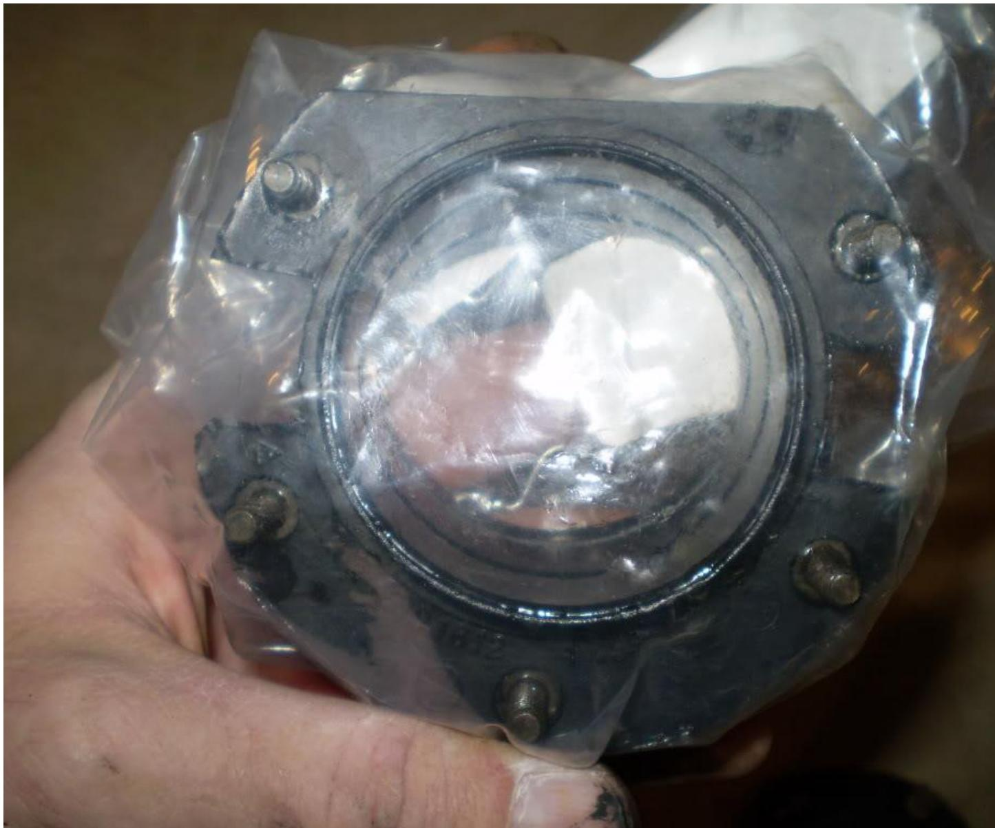
You can see the bits and pieces of nasty black tar-gunk in the fuel pump strainer basket and in the bottom of the tank-- the hole you see is where the fuel pump assembly sits. Until I pulled the pump assembly today, I didn't realize the strainer basket was in such bad shape (note the gunk AND the holes in the woven material), so I still need to call the dealer and order another one.
