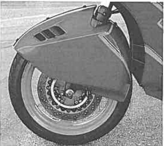
Top to bottom: The K1 bristles with unique touches including fairing-mounted switches and gauges; the rear seat cowl comes off for two-up riding; single-shock Paralever controls driveshaft effect; front wheel cowl improves aerodynamics.
