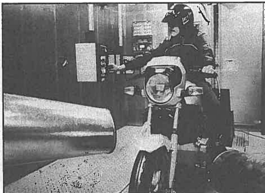
Each machine is tested on rollers before it leaves the factory.
