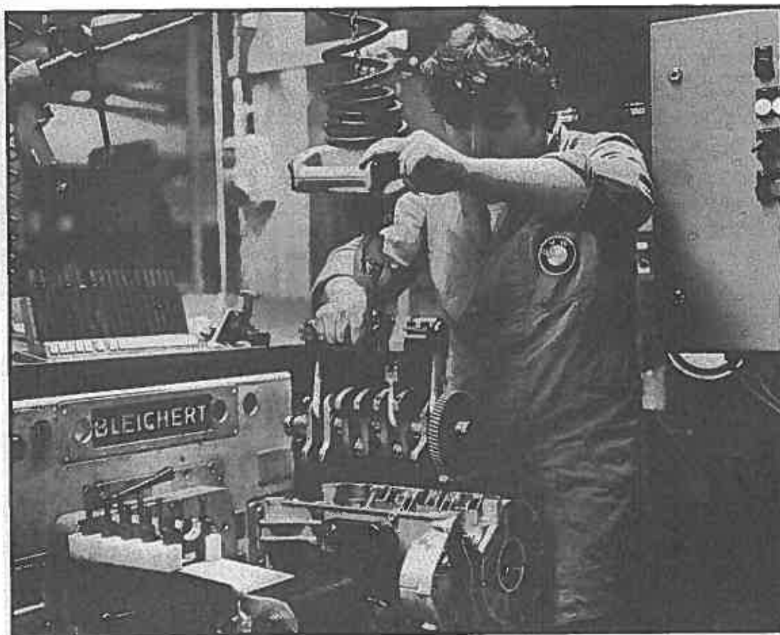
Far left: Bikes rest on suspended platforms as they travel along the 1.2 kilometre-long assembly line. Each model has a code number, and by entering this in the central computer, it can be sent along the correct path and will stop at the necessary assembly stations. Left: On the engine assembly line, a K series crankshaft is installed in its housing.
