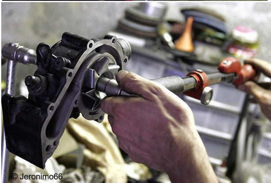
Replace the O ring on the small pinion
