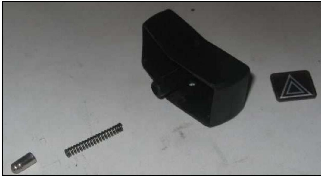
**(Optional)** If the graphic insert on the switch is worn (because you're a wimp and use your heated grips all of the time) you can push it out from the inside. A replacement can be had from BMW for about \$4-5. They just pop right back in and make the switch look brand new again.
