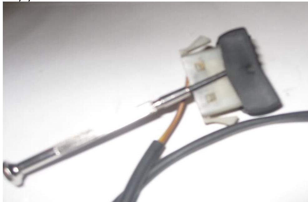
This is the step where you can lose tiny bits. In the rocker is a little tube holding a spring and a little part at the end which, when translated into English by German engineers, is called the little hollow phallus.
