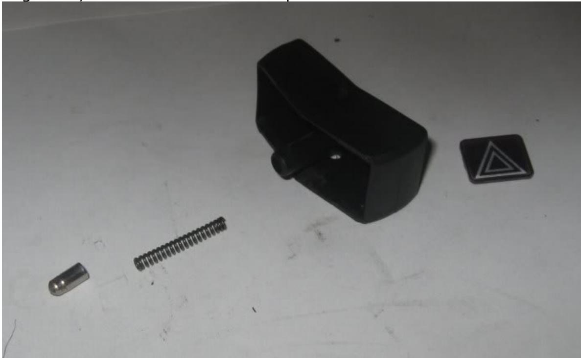
(Optional) If the graphic insert on the switch is worn (because you're a wimp and use heated grips all of the time) you can push it out from the inside. A replacement can be had from BMW for about \$4-5. They just pop right back in and make the switch look brand new again.
