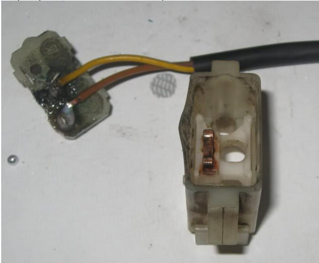
Step 11) Put the rocker back on. Before you do, use a pen or something to get the slider in a halfway position. Put the rocker on its back (otherwise the little hollow phallus will escape) and push the switch straight into it.
