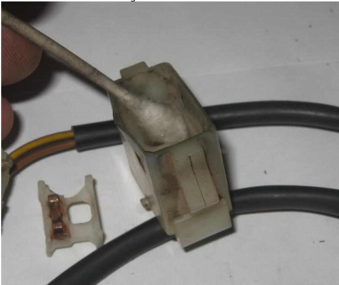
Also do the upper outside of the switch body and the inside of the rocker.
