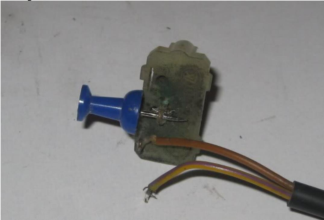
Step 9) Cut the old end of the wire off and strip about 1/4 inch. Put it through the hole and solder it back on.
