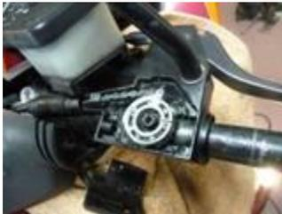
Apply a moderate amount of general purpose lithium grease to moving parts, the handlebar sleeve and inside cam housing.
