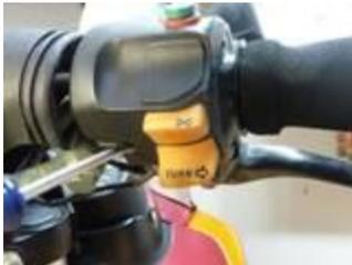
Remove throttle gear cover. Note the two indexing marks aligning cam gear and twist grip.
