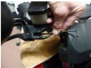
Now the throttle cam gear and twist grip can be removed after decoupling throttle cable from chain fitting.
