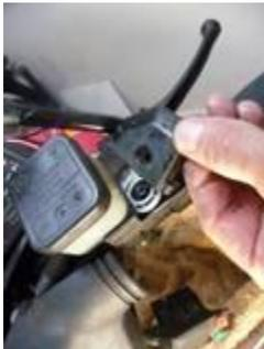
Unscrew the two 4 mm hex screws holding brake master cylinder to handgrip assembly. Slide m/c gently toward steering head. You are keeping that upright, right?
