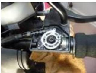
Slide throttle grip onto bar and align with cam using the index marks. Carefully slide m/c assembly into position, making sure m/c piston slides into brake-lever housing. Snug up m/c with two hex screws (it's easier if you thread rearmost screw first). Install throttle cam housing cover, then switch cover. Clean up greasy paw prints so your customer is happy with the result.>
